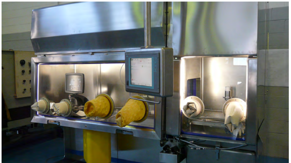
> 1. Isolator module with integrated incubator
