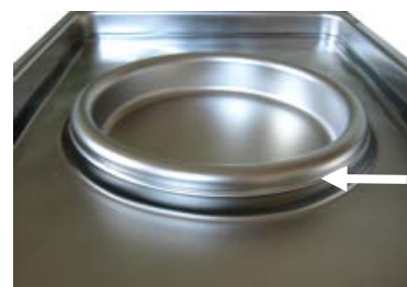
Figure 14: Incubators size 170 / 260, Filling height line of the outer basin
