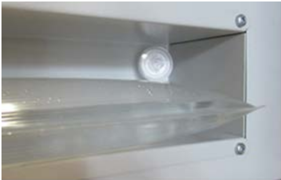
Figure 52: Location of the gas fine filter (sterile filter) in the recess for the freshwater bag
