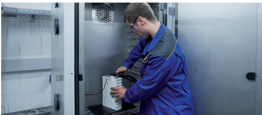
› Endurance testing of cells and modules under simulation of changing environmental influences
