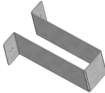
Figure 9: Spacer for wall distance
