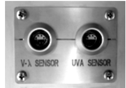
Figure 14: Lemo sockets to connect the light sensors
