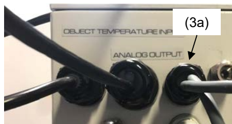
Figure 31: Connection cable on the "Object temperature input" connection (3a)
