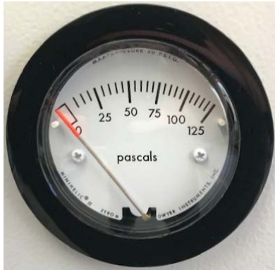
Figure 24: Analog pressure display (manometer) for monitoring the compressed air flushing on the chamber front
