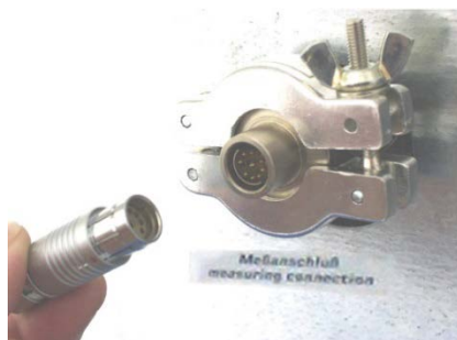
Figure 30: Measuring connection (12) with measuring access port
