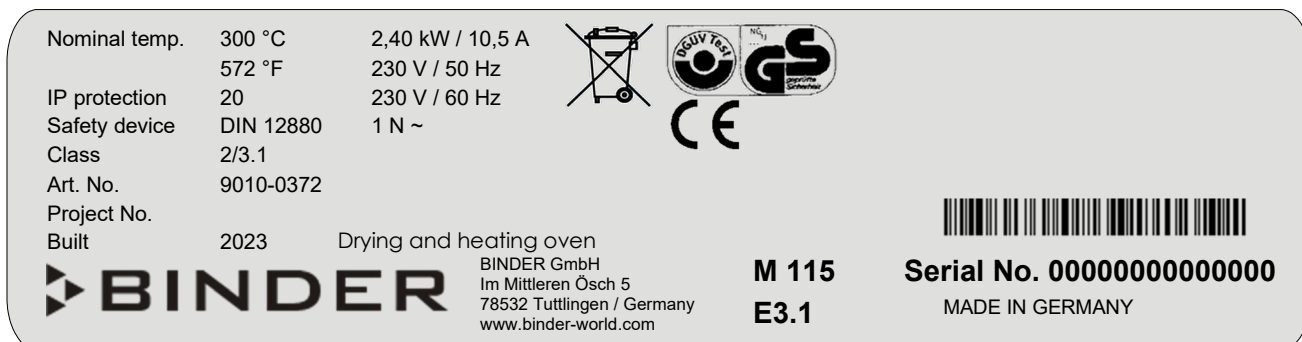
Figure 2: Type plate (example M 115 regular chamber)
