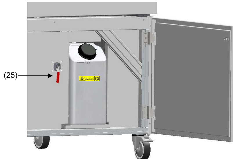
Figure 12: Lever for condensate recycling (open position) next to the freshwater can behind the maintenance access door
