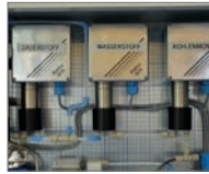
CO, H 2 , and O 2 are detected and monitored in the testing area atmosphere
